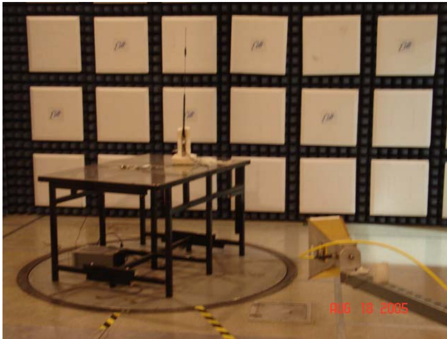
Test Setup for Radiated Emissions with the Omni Antenna - Horizontal Polarization
