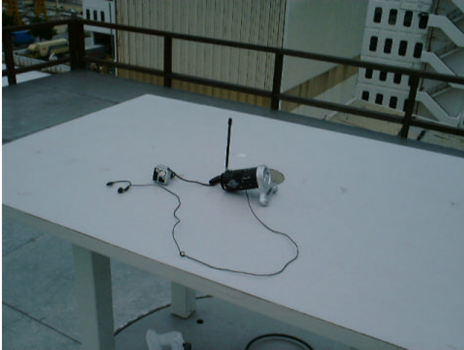
Measurement of Radiated Emission Test Set Up
