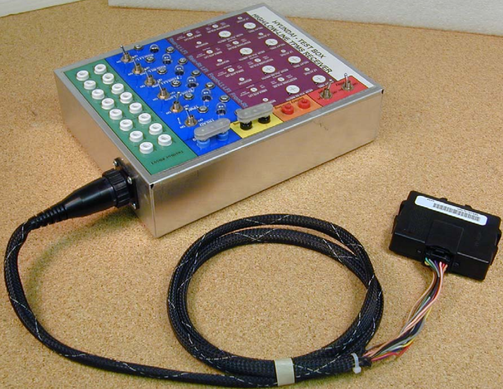
DUT with Harness and Load Box
