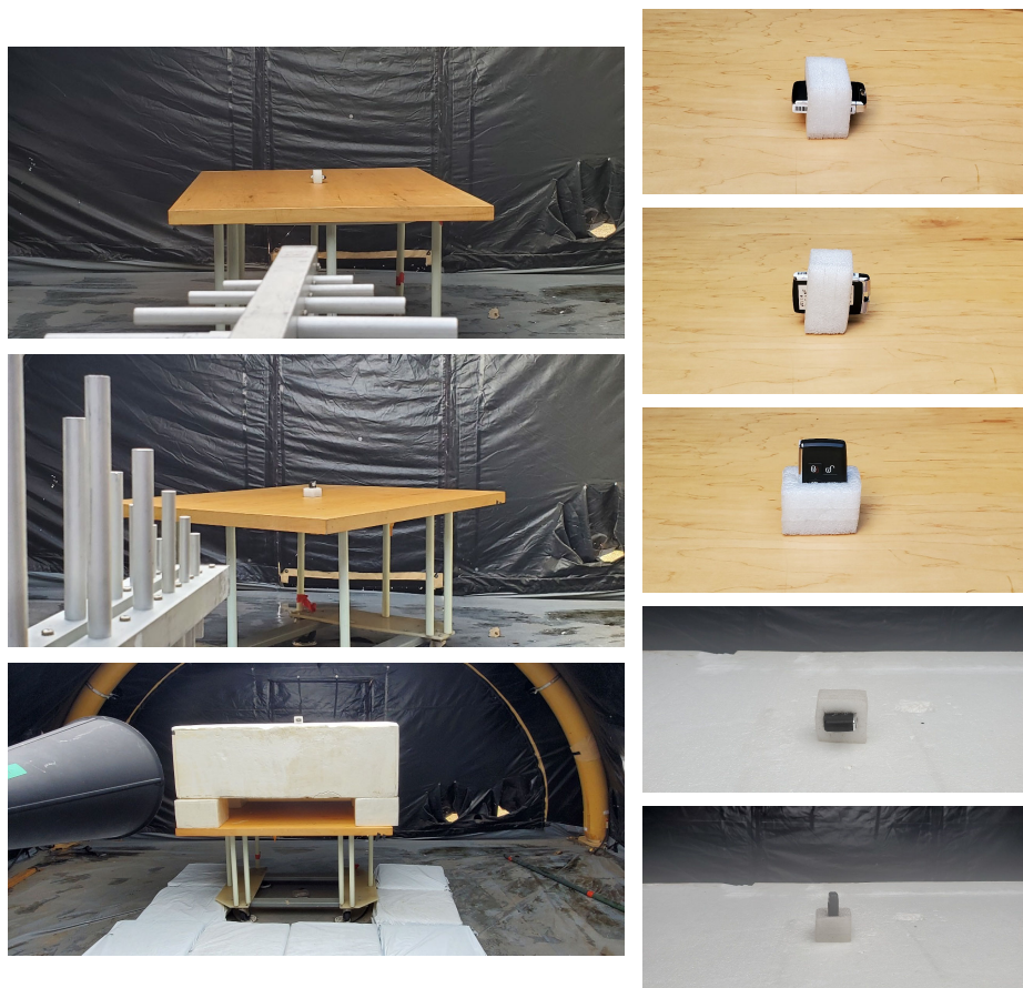
Figure 4: Radiated Emissions Test Setup Photograph(s).
