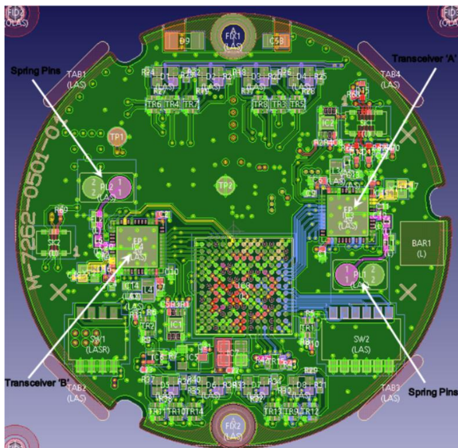
Figure 2. Main PCB showing Transceiver and Spring Pin positions
