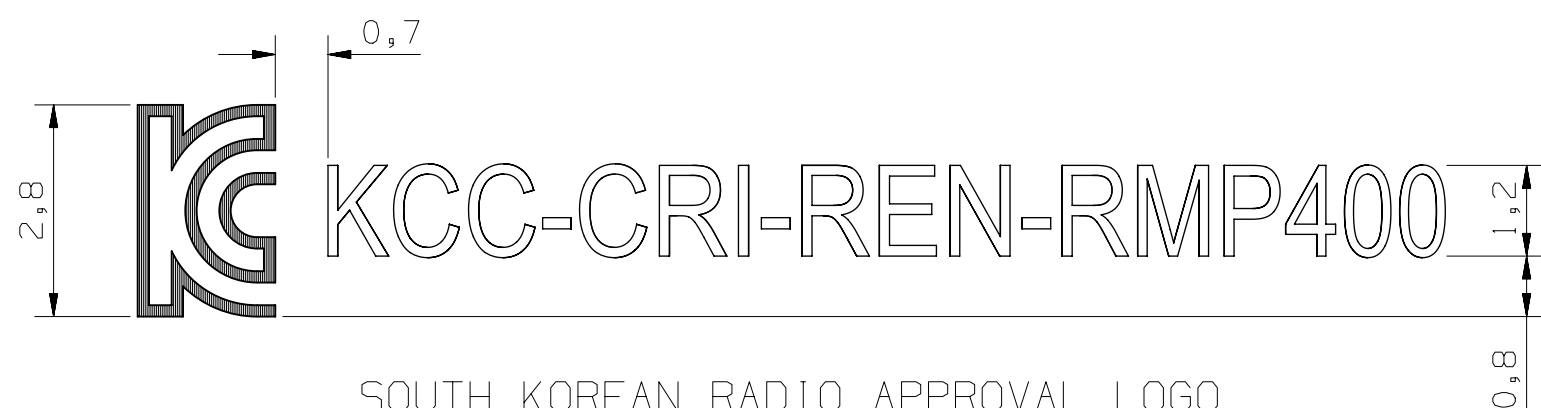
SOUTH KOREAN RADIO APPROVAL LOGO TO BE HORIZONTALLY CENTRAL TO PART CENTERLINE
