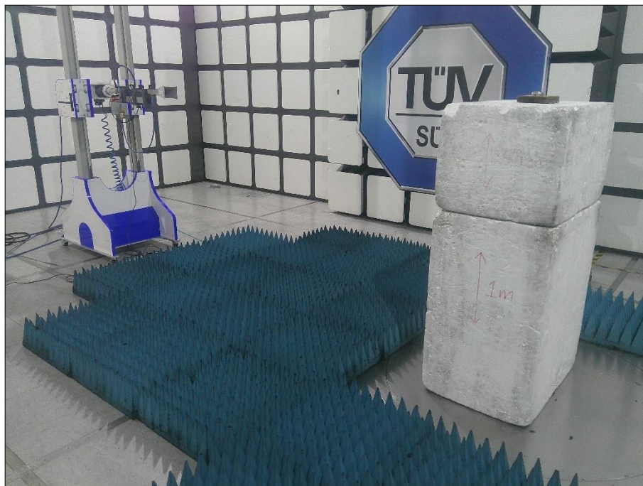
Figure 58 - Test Setup - 8 GHz to 18 GHz
