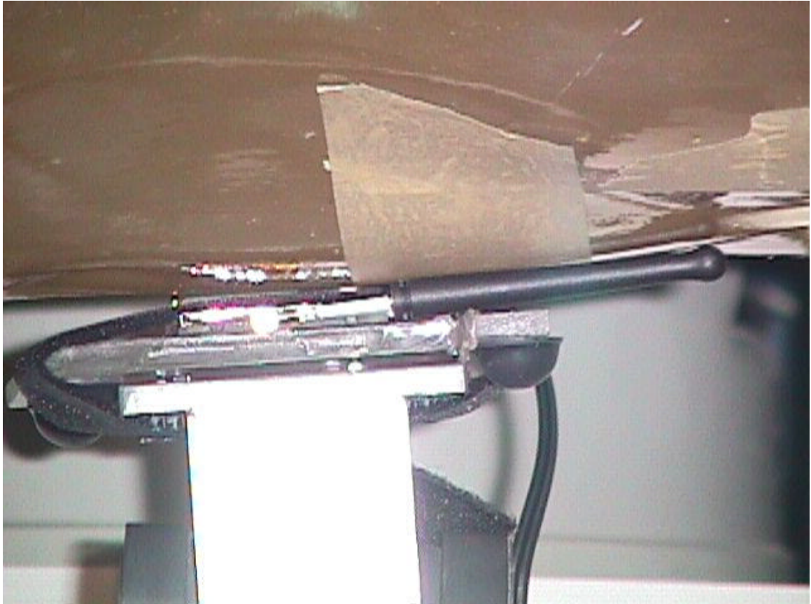
< Waist with the Centurion, WCP-2400-MMCX 1/4 wave dipole antenna, 10mW unit – Close-up view >
