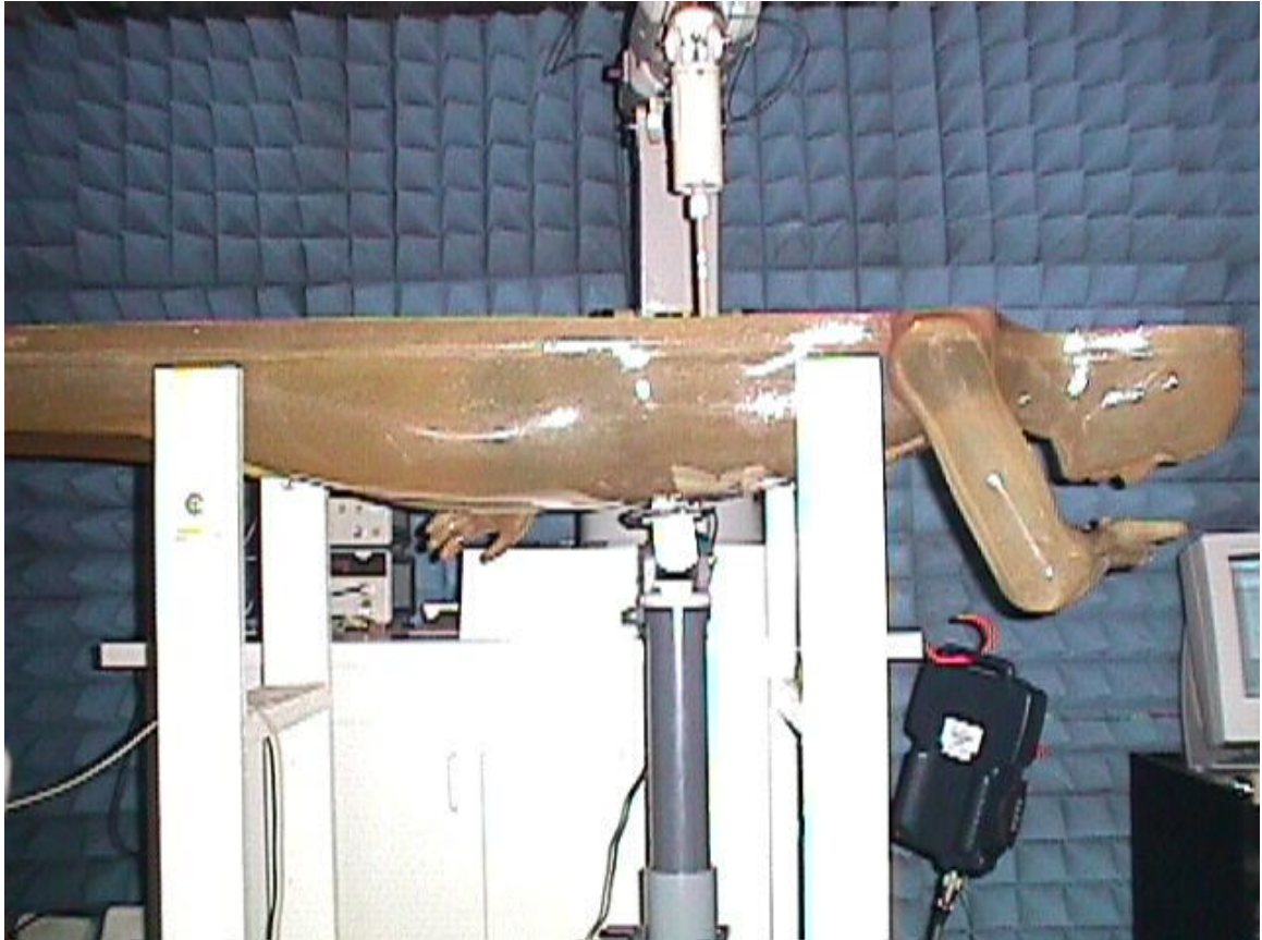
< Waist with the Centurion, WCP-2400-MMCX ¼ wave dipole antenna, 10mW unit – Overview >
