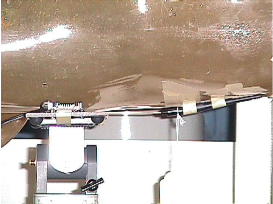
< Waist with the Nearson, S181FL-5-RMM-2450S \frac{1}{4} wave dipole antenna, 10mW unit – Close-up view >
