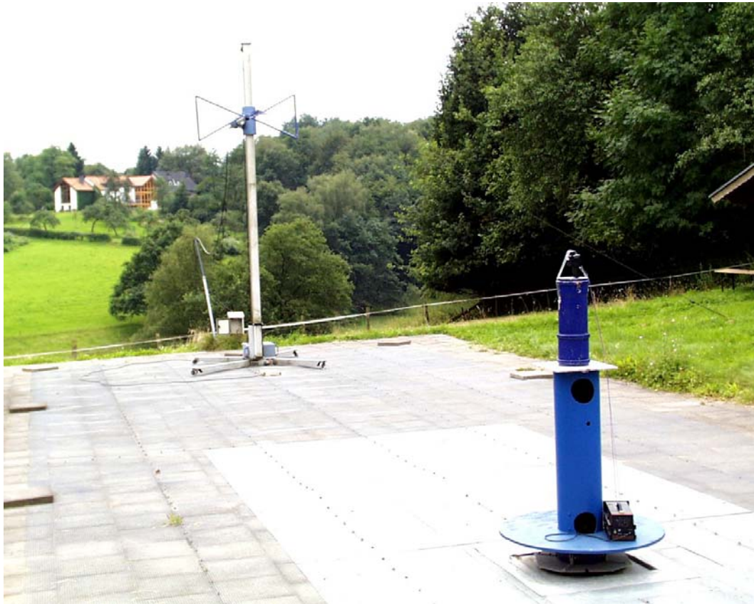
Photographs of Test Setups (Spurious measurements) EUT : Siemens VDO 5WK4 7631
