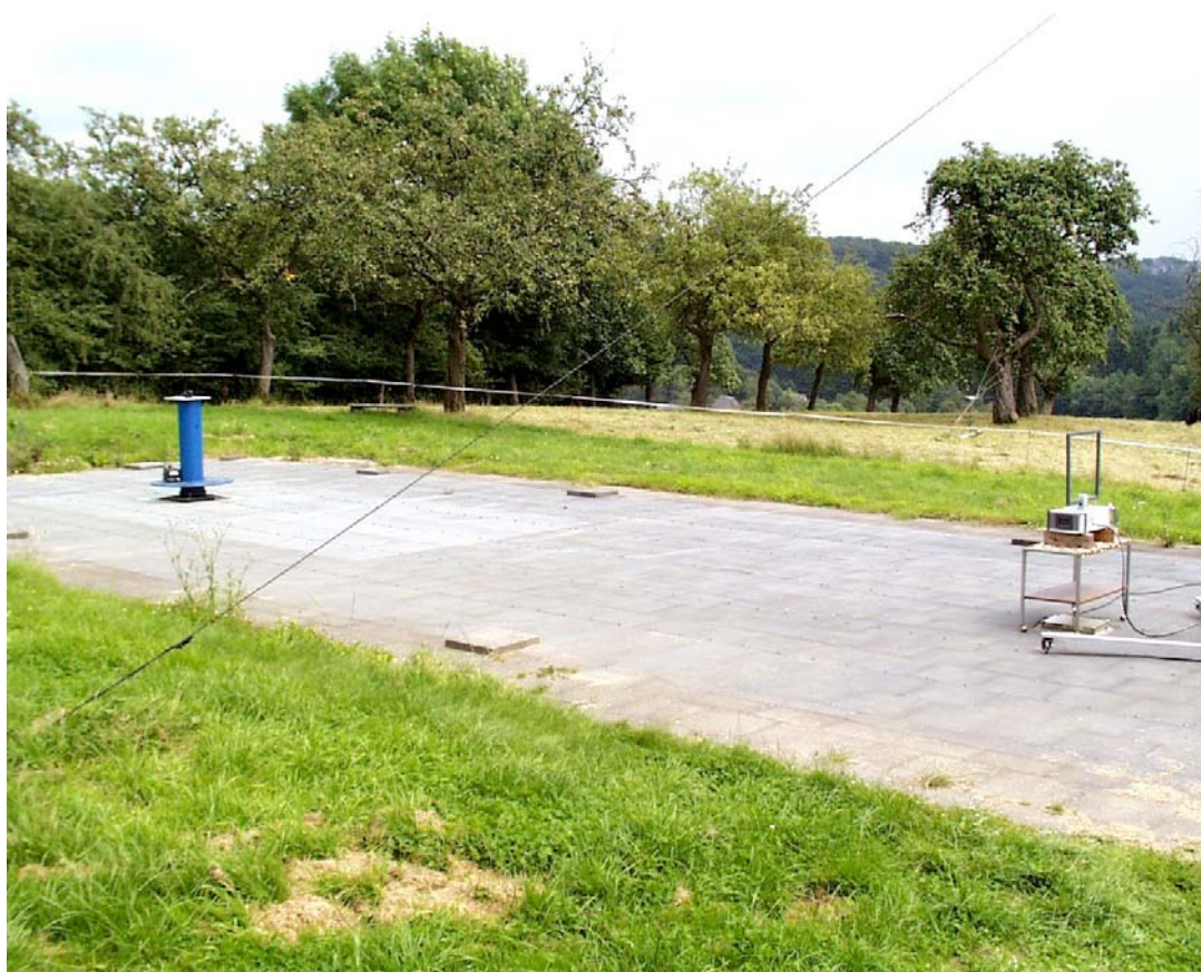
Photographs of Test Setups (Inductive application measurements) EUT : Siemens VDO 5WK4 7631
