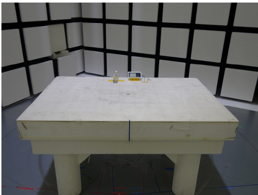
Photograph 2: Set-up for Radiated Spurious Emission below 30MHz, Front View
