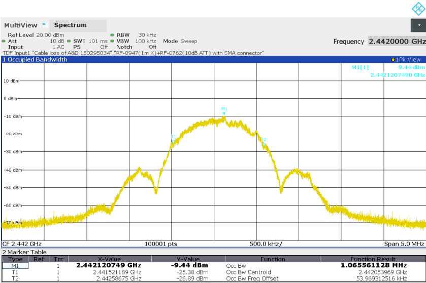
Figure 9: 99% Bandwidth, BLE, Mode M (2442MHz), 1Mbps
