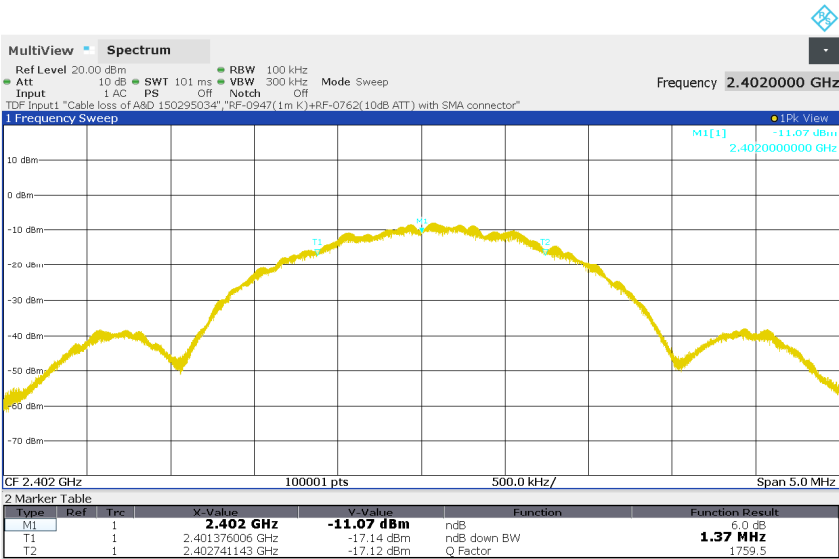
Figure 5: 6dB Bandwidth, BLE, Mode L (2402MHz), 2Mbps
