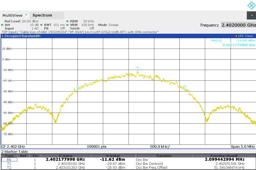
Figure 11: 99% Bandwidth, BLE, Mode L (2402MHz), 2Mbps
