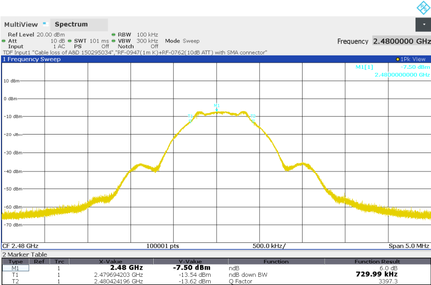
Figure 4: 6dB Bandwidth, BLE, Mode H (2480MHz), 1Mbps
