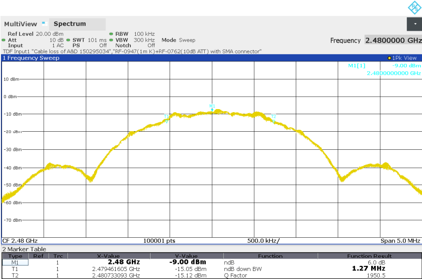
Figure 7: 6dB Bandwidth, BLE, Mode H (2480MHz), 2Mbps
