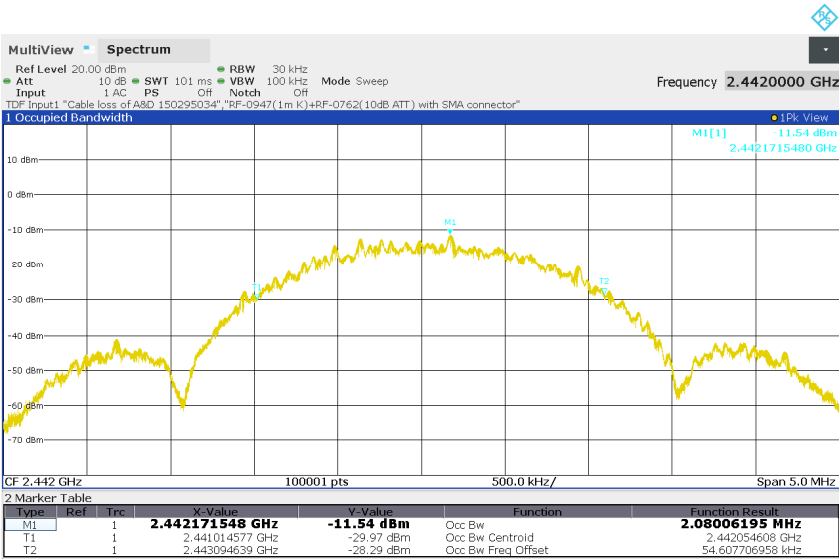
Figure 12: 99% Bandwidth, BLE, Mode M (2442MHz), 2Mbps
