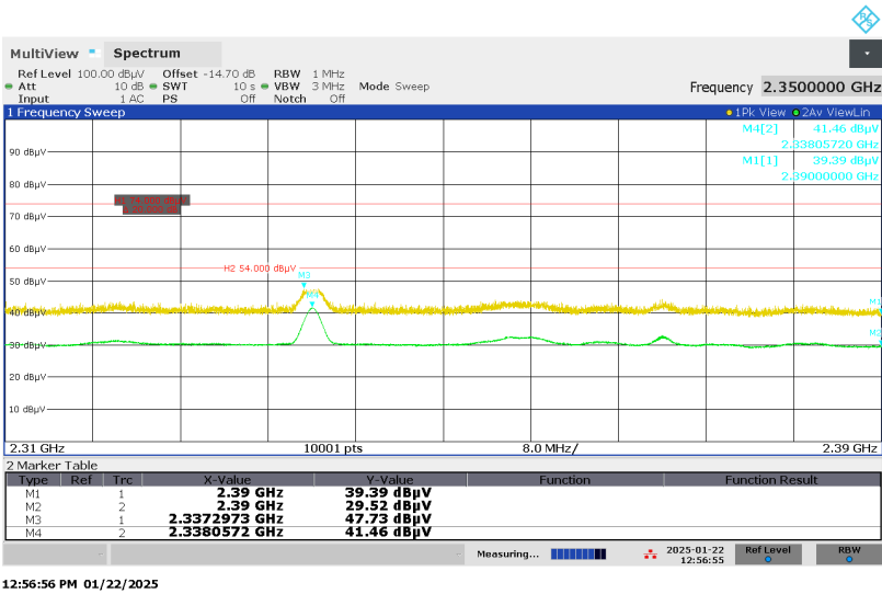
Figure 35: Restricted-band Band-edge, Spectral Diagram, Vertical Antenna Orientation, BLE, Mode L (2402MHz), 2Mbps
