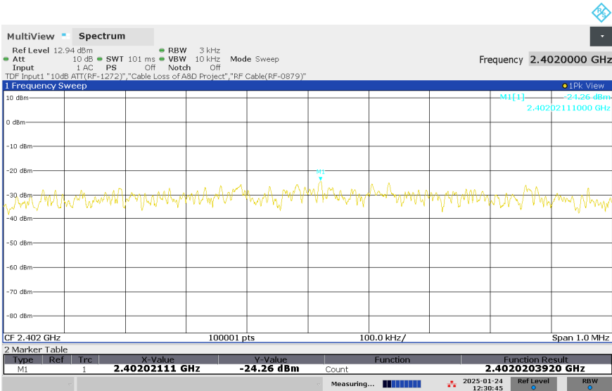
Figure 27: Power Spectral Density, BLE, Mode L (2402MHz), 2Mbps
