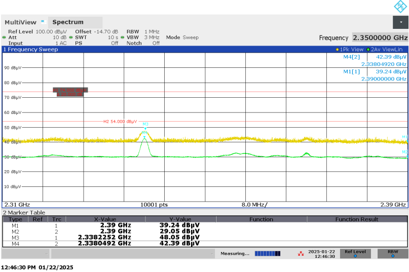
Figure 31: Restricted-band Band-edge, Spectral Diagram, Vertical Antenna Orientation, BLE, Mode L (2402MHz), 1Mbps
