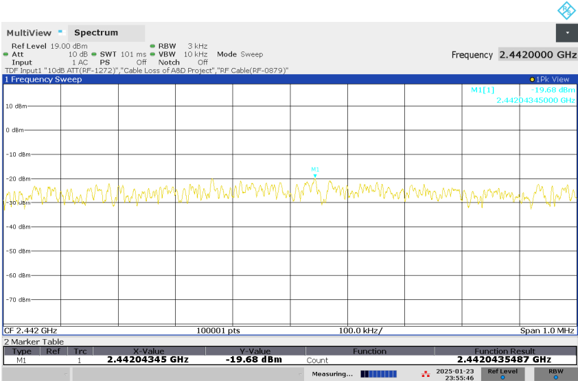
Figure 28: Power Spectral Density, BLE, Mode M (2442MHz), 2Mbps
