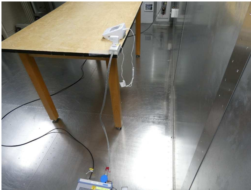
Photograph 8: Set-up for AC Power Line Conducted Emission, Rear View
