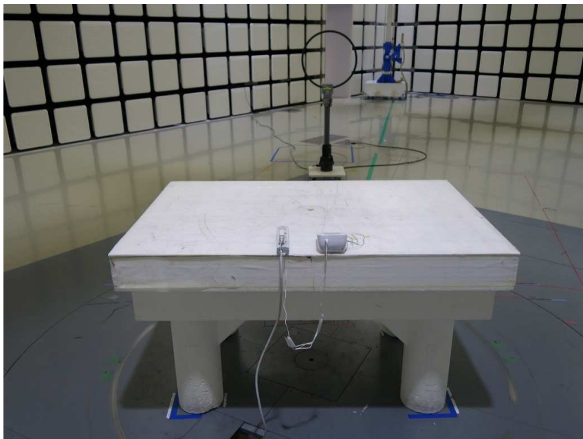
Photograph 2: Set-up for Radiated Spurious Emission below 30MHz
