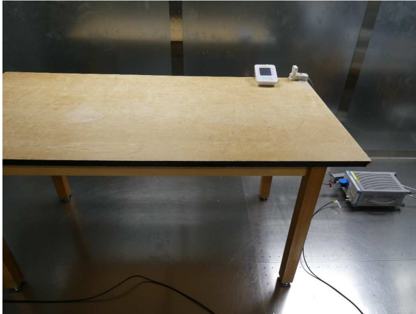
Photograph 7: Set-up for AC Power Line Conducted Emission, Front View
