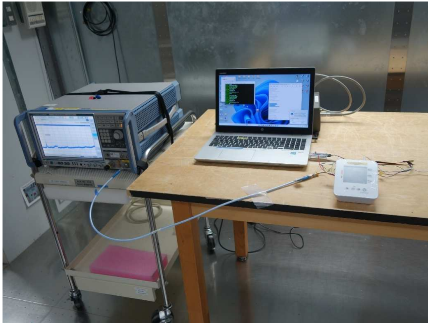
Photograph 1: Set-up for Antenna Port Conducted Emission of Transmitter, General View
