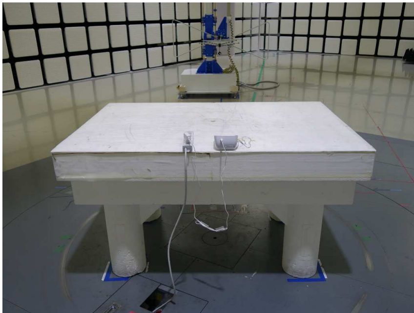
Photograph 4: Set-up for Radiated Spurious Emission below 1GHz, Rear View
