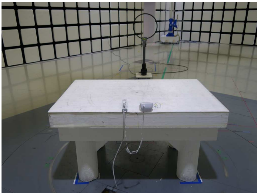
Photograph 2: Set-up for Radiated Spurious Emission below 30MHz
