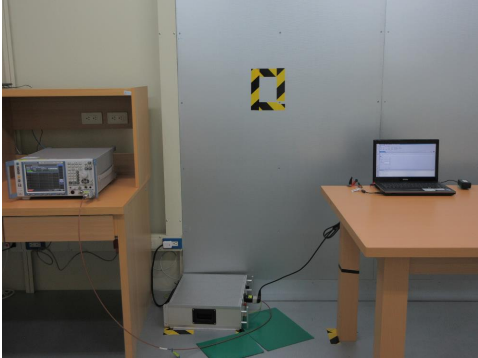
Photograph 7: Set-up for AC Mains (Front View)
