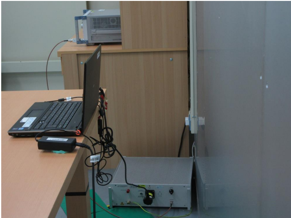
Photograph 8: Set-up for AC Mains (Back View)
