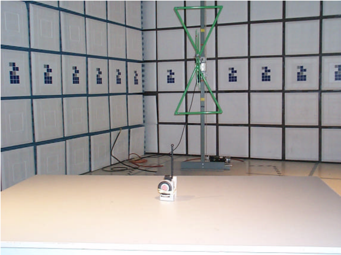
Maximized Radiated Emission Test Set-up Vertical Polarization
