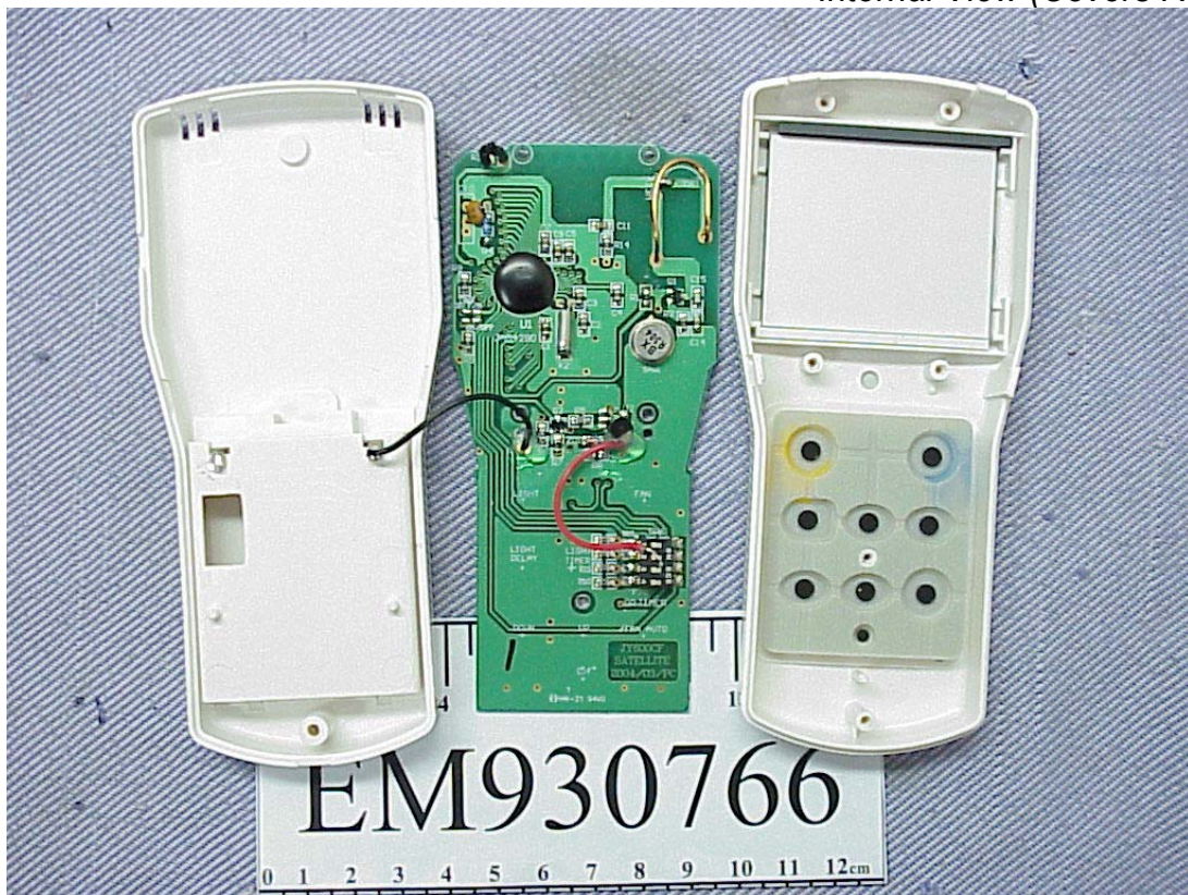
Photos 5 P. C. Board View (Component Side)
