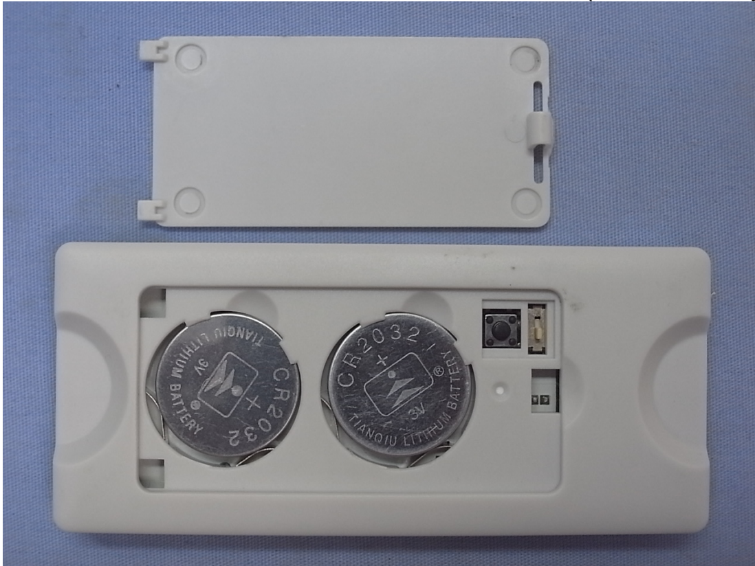
Photo 6 Internal View (Removed Battery Cover)
