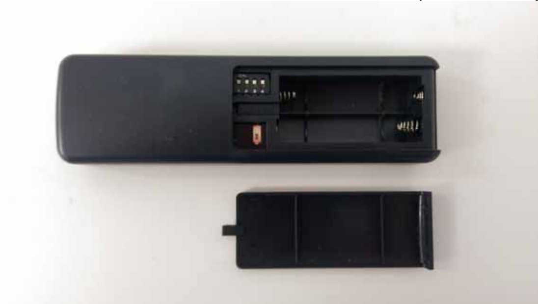
Photo 3 Internal View (Removed Battery Cover)
