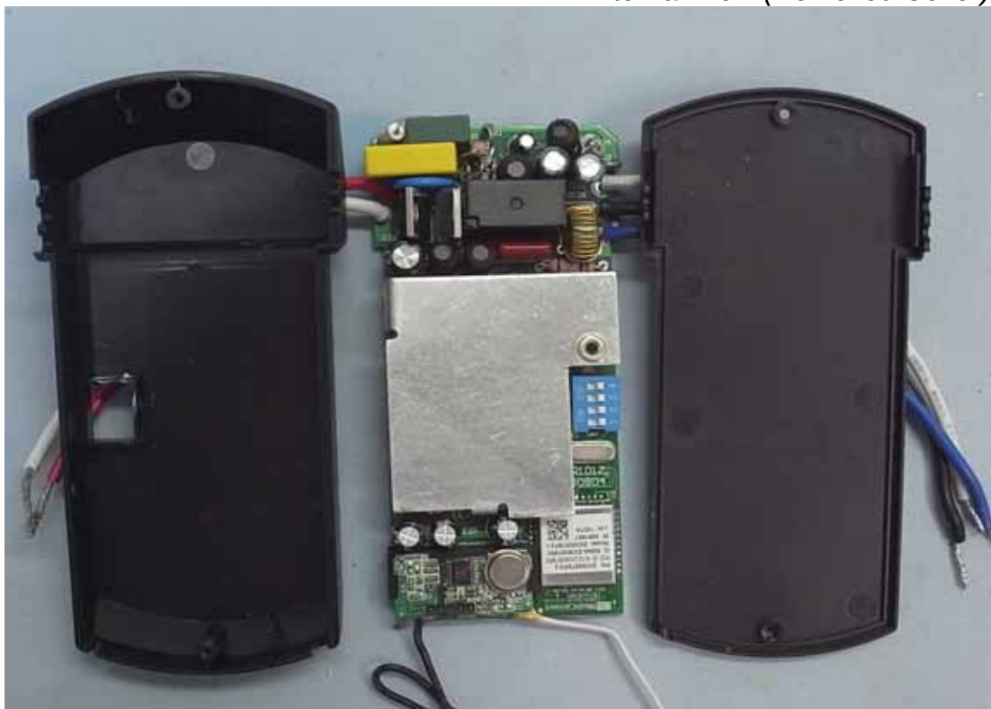
Figure 4 Internal View (Removed Cover)
