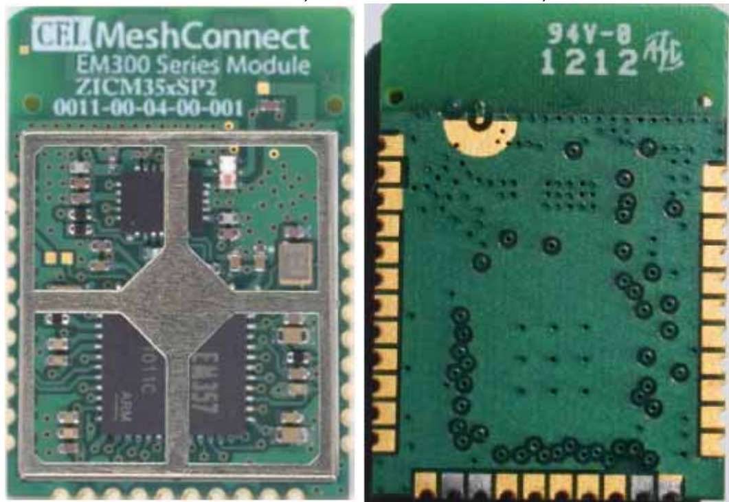
Figure 10 RF Module, Removed Shield Cover, Front & Back View
