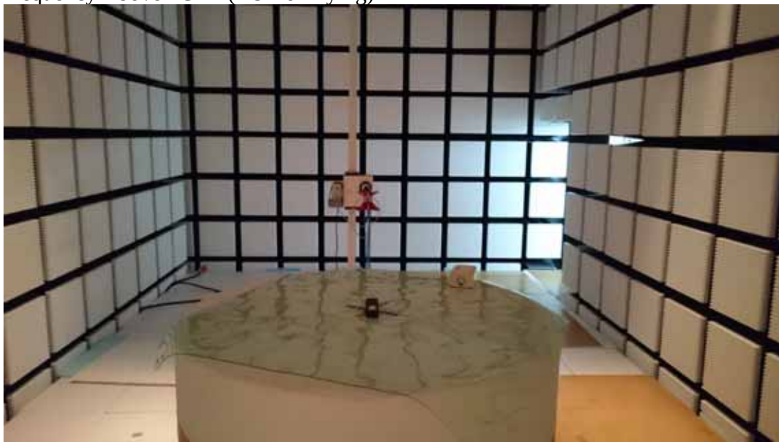
Frequency Above 1GHz (EUT on Lying)
