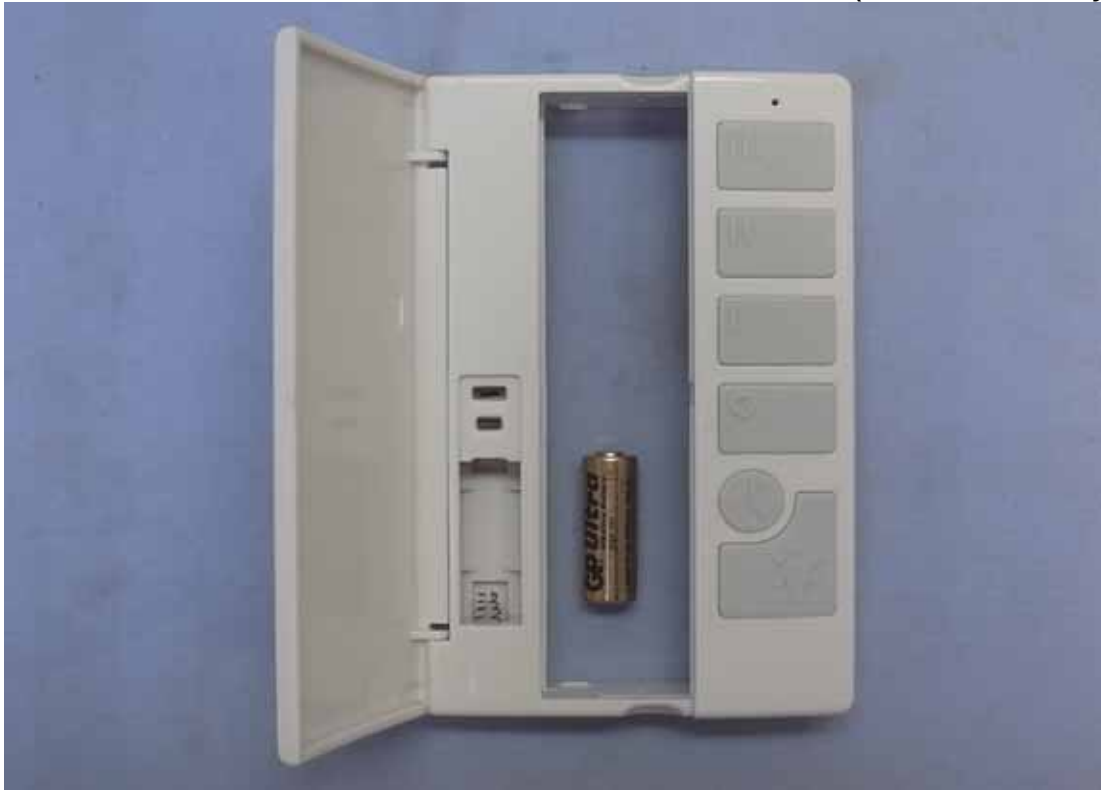
Photo 3 Internal View (Removed Battery Cover)
