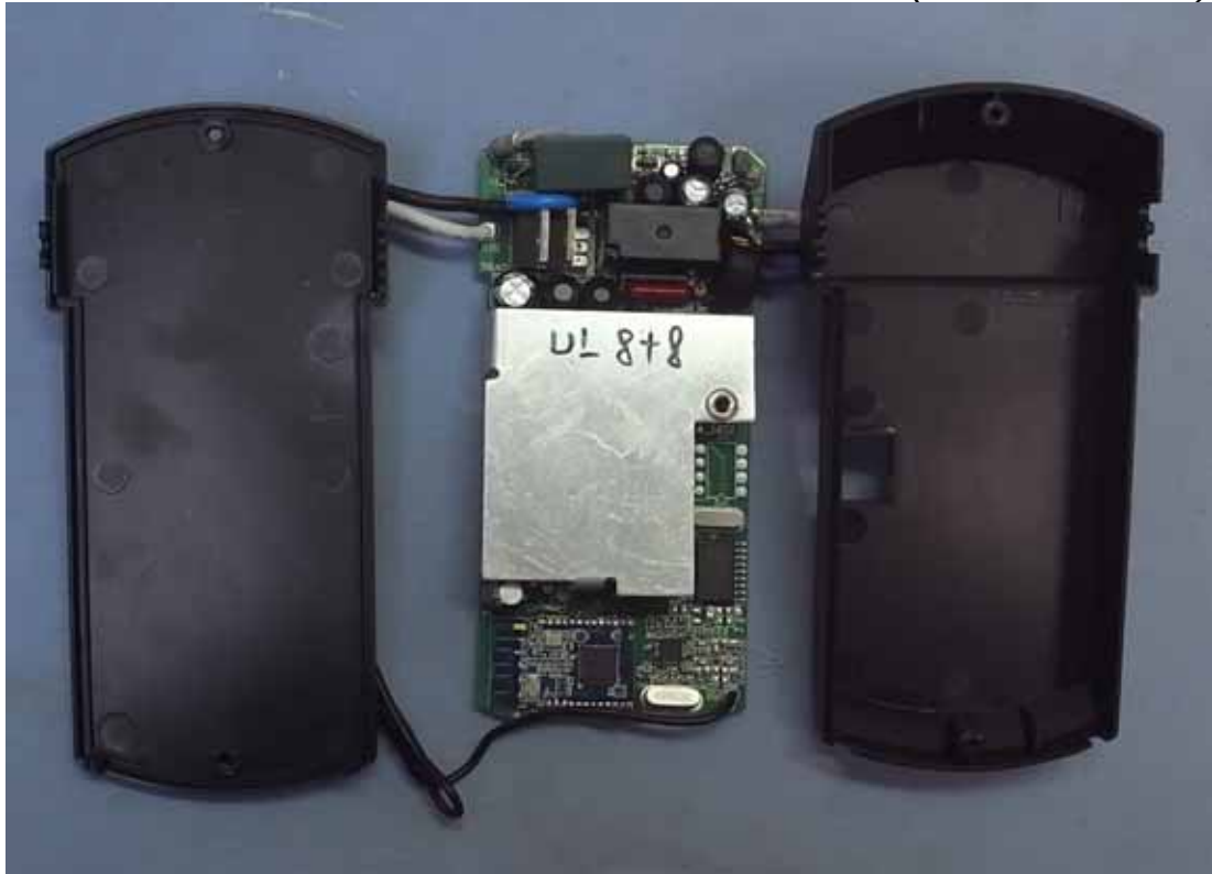
Figure 4 Internal View (Removed Cover)
