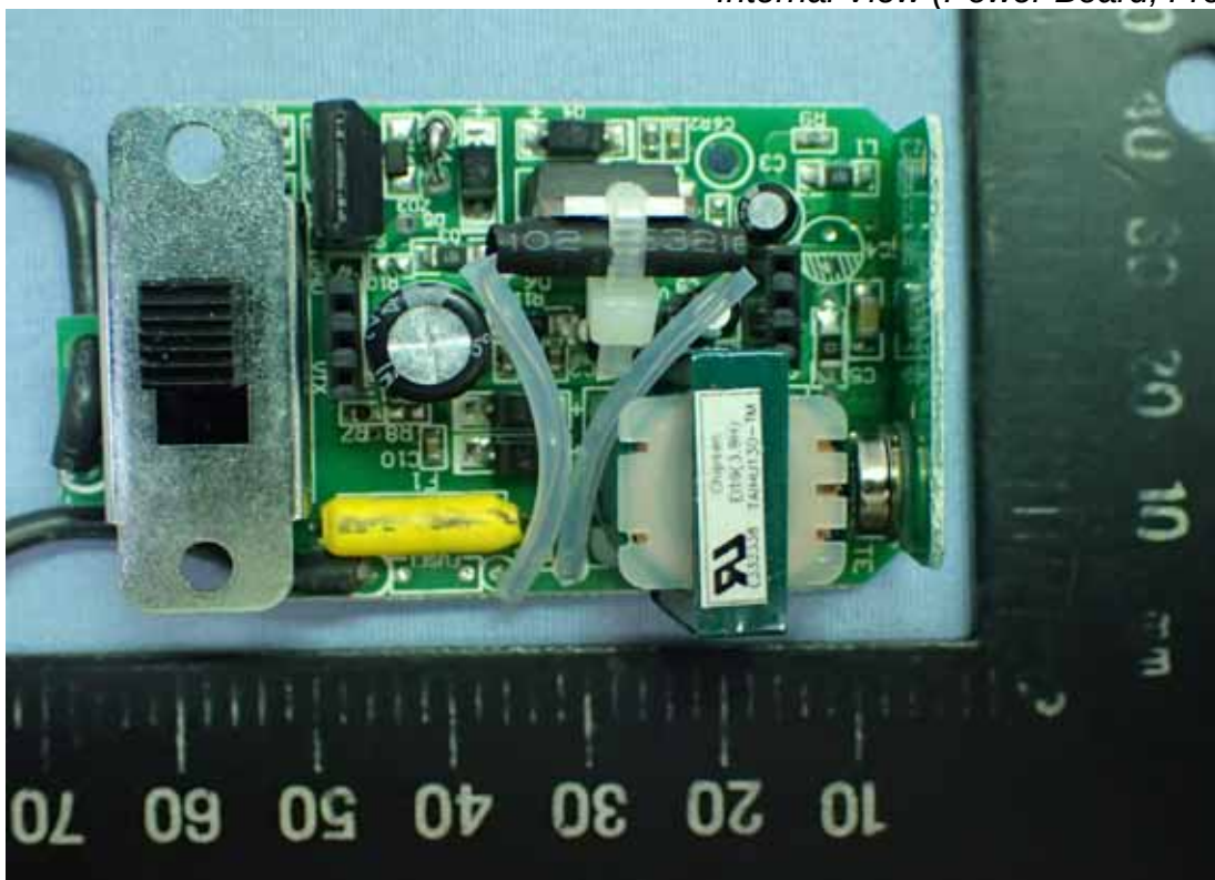
Photo 6 Internal View (Power Board, Front View)
