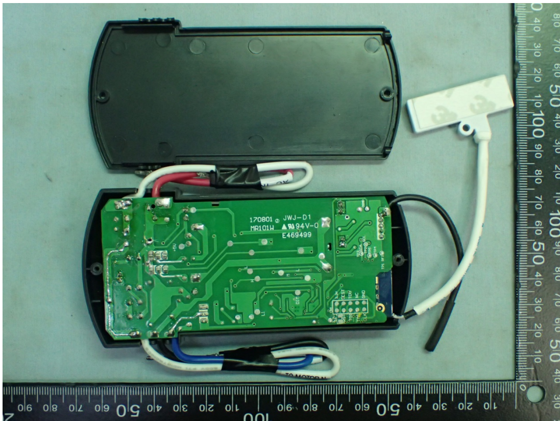
Figure 3 Internal View (Removed Cover)
