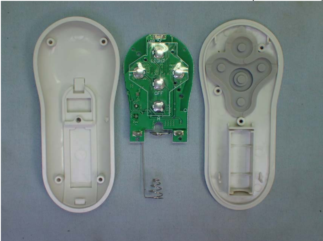
Figure 4 Internal View (Removed Cover)
