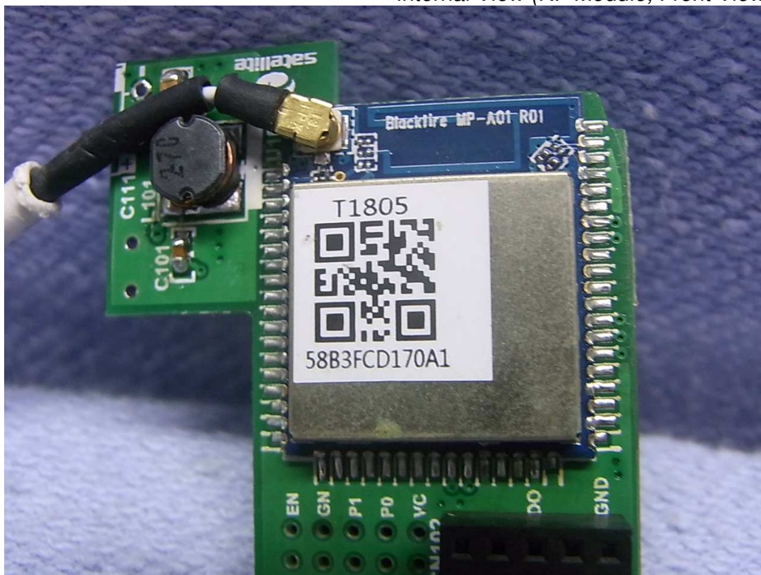
Figure 8 Internal View (RF Module, Front View)
