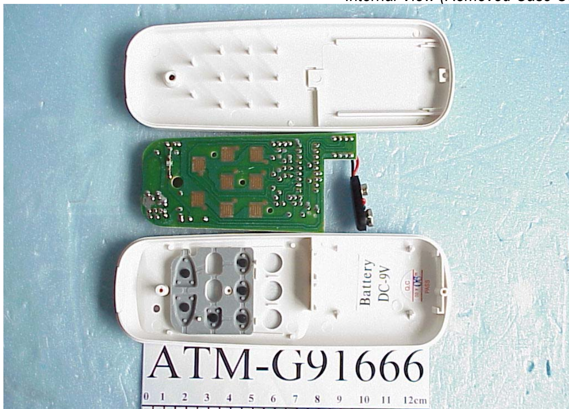
Photos 3 Internal View (Removed Case Covers)
