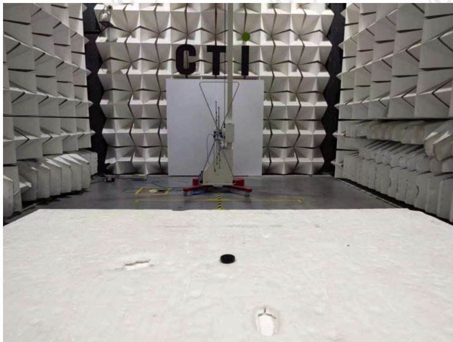
Radiated emission Test Setup-1 (30MHz~1GHz)
