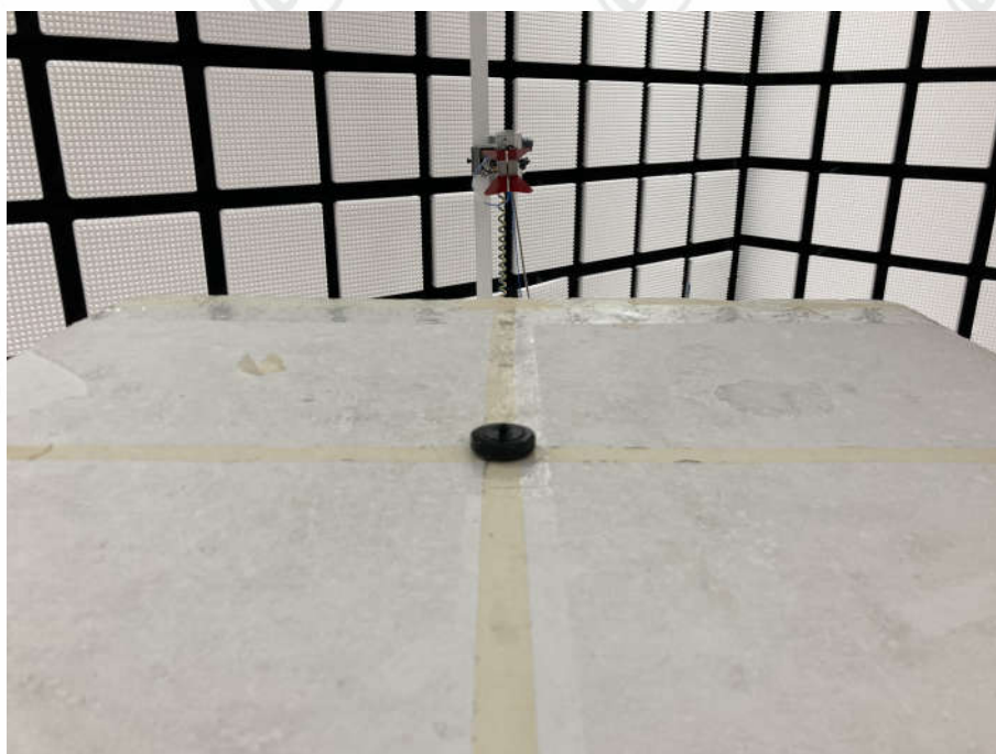
Radiated spurious emission Test Setup-2 (Above 1GHz)
