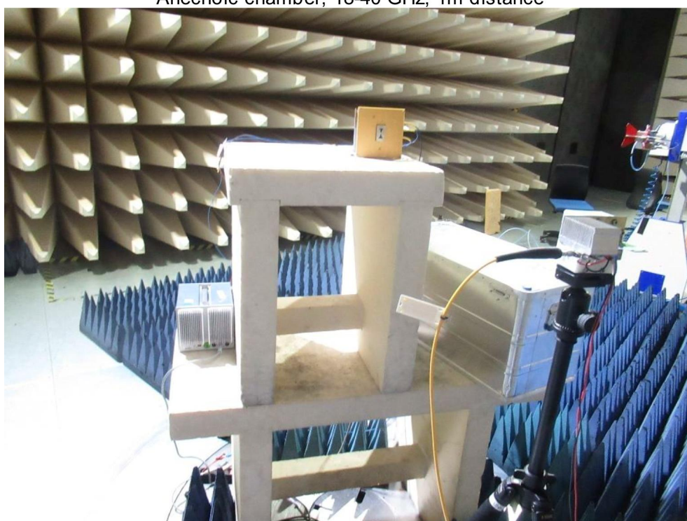
Anechoic chamber, 18-40 GHz, 1m distance
