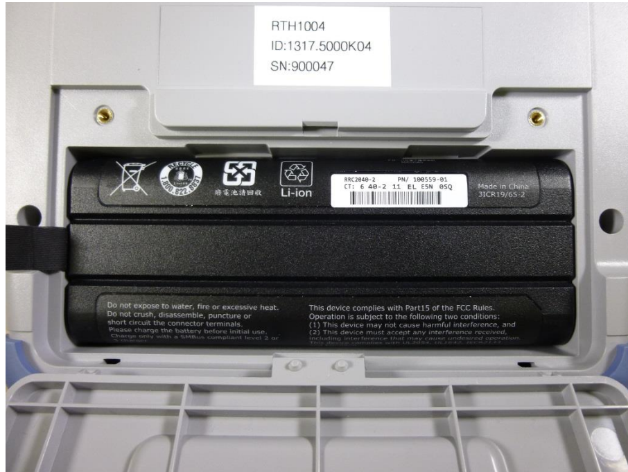
Photo 11: Battery box with battery
