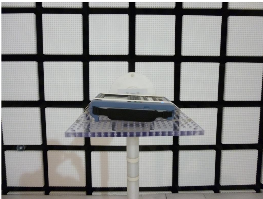
Photo 5: Fully anechoic chamber
