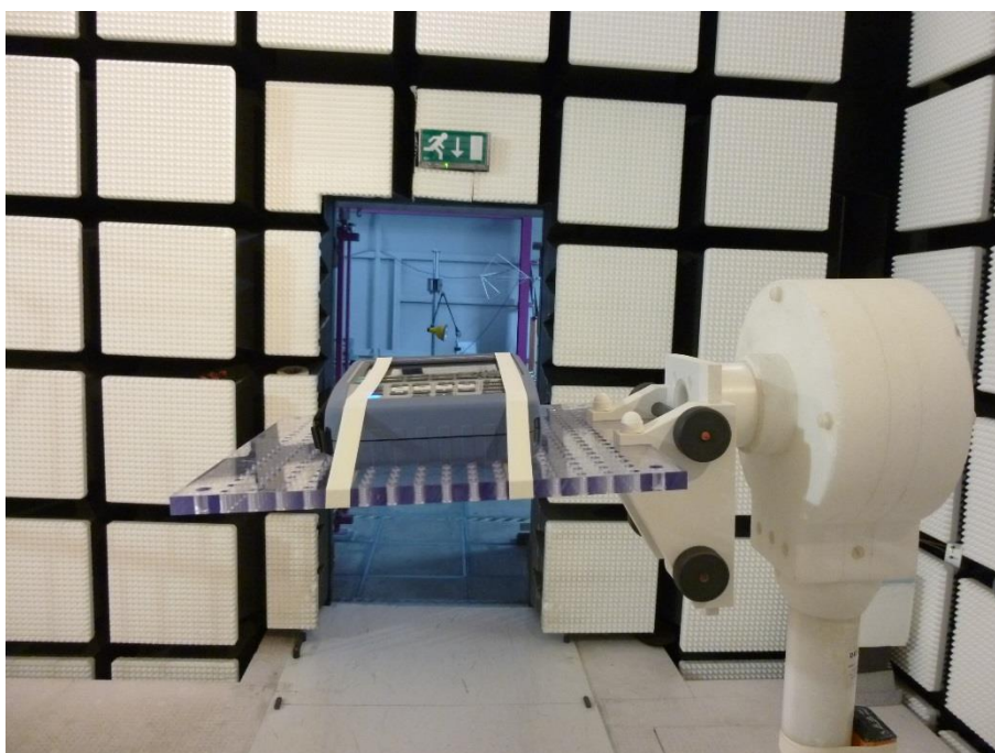
Photo 6: Fully anechoic chamber
