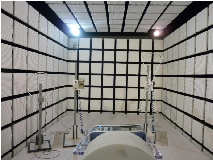
Photo 7: Fully anechoic chamber
