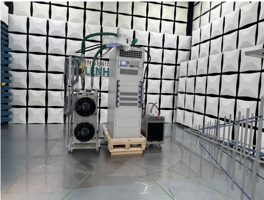
Photograph 4: Overall view 2. Radiated cabinet measurement with signal power on EUT 2 kW. The door of the chamber is closed. The power supply is provided through the socket in the turn table.
