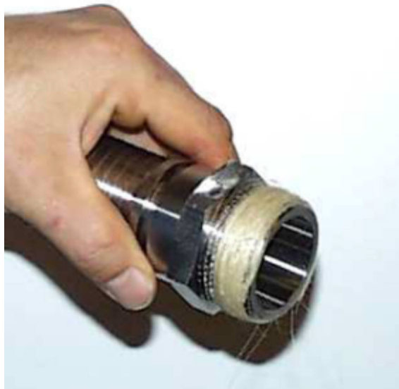
Figure 4-43: Finished hemp packing.
