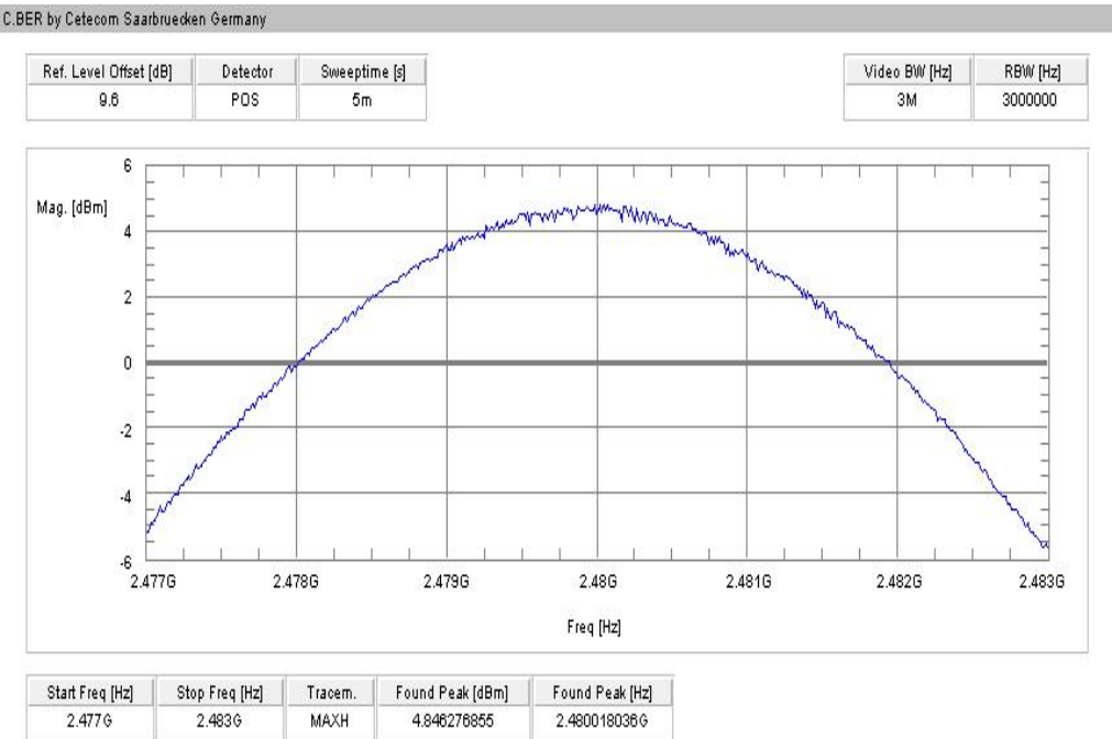
Plot 9: highest channel – 2480 MHz, 8 DPSK modulation
