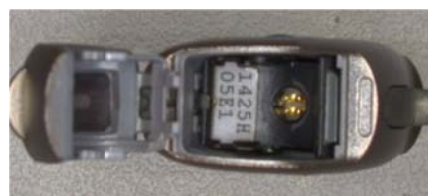
Figure 2: Phonak Audeo V battery compartment, current serial number size is about 2 points
