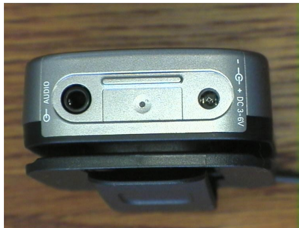
fig. 7 Campus S back view (left audio input, right DC charger input)
