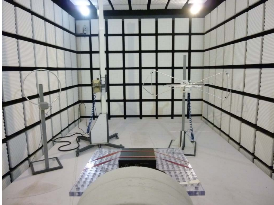
Photo 3: Anechoic chamber test setup
