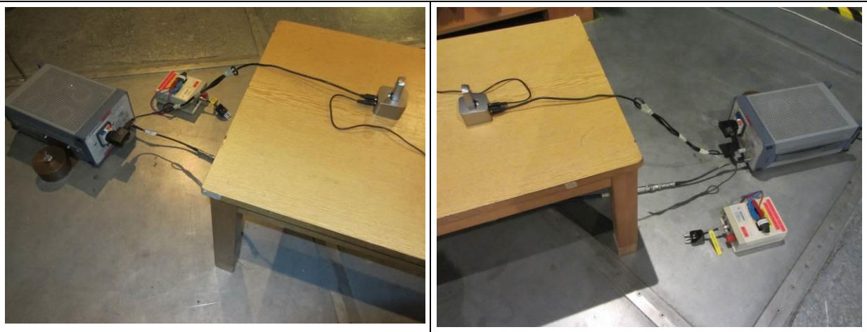
Fig 1 Conducted measurements – interference voltage
