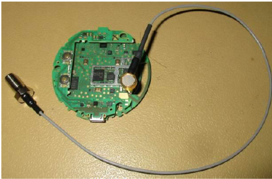
Electronic board with temporary antenna connector
