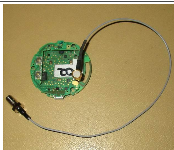
Electronic board with temporary antenna connector
