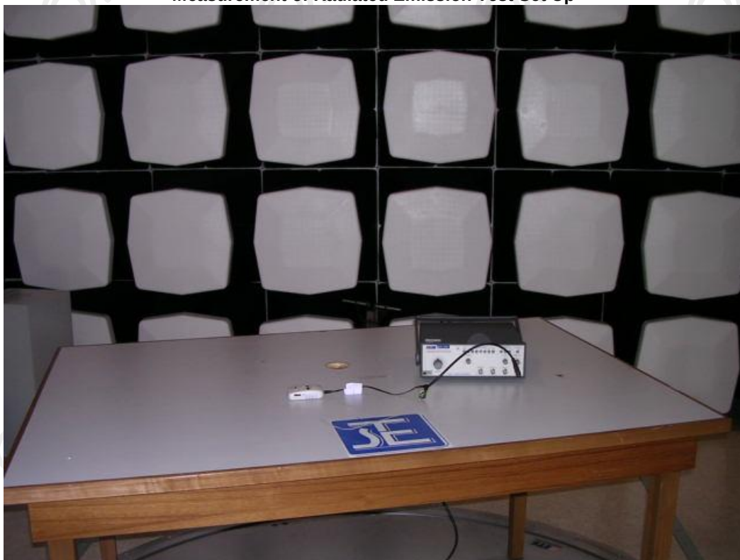
Measurement of Radiated Emission Test Set Up
