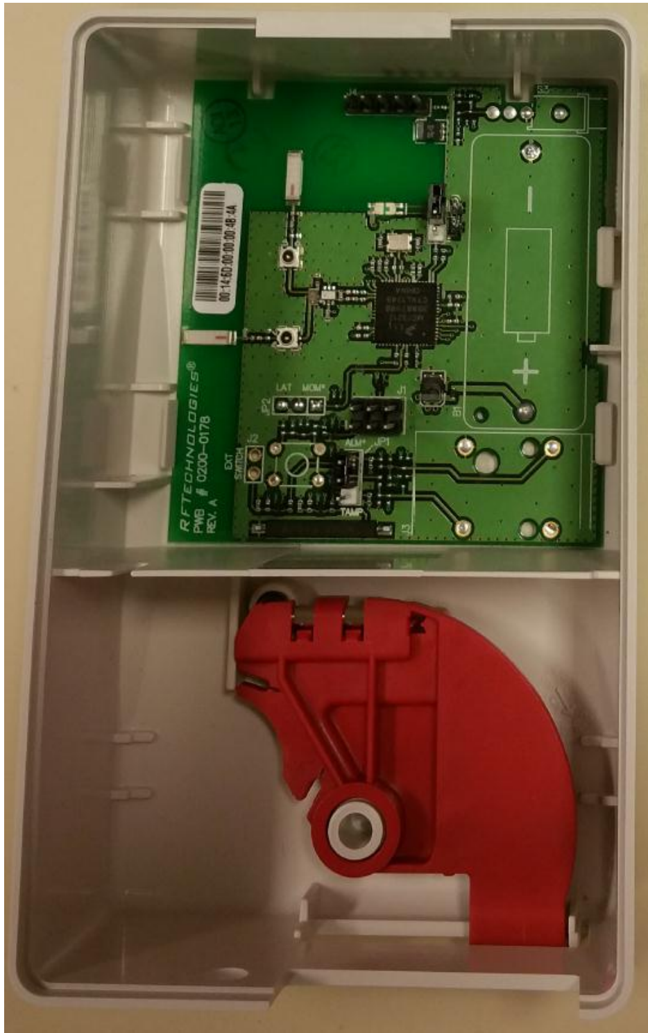
Model 0800-0539 Inside Main Unit & Built In Battery Pack
