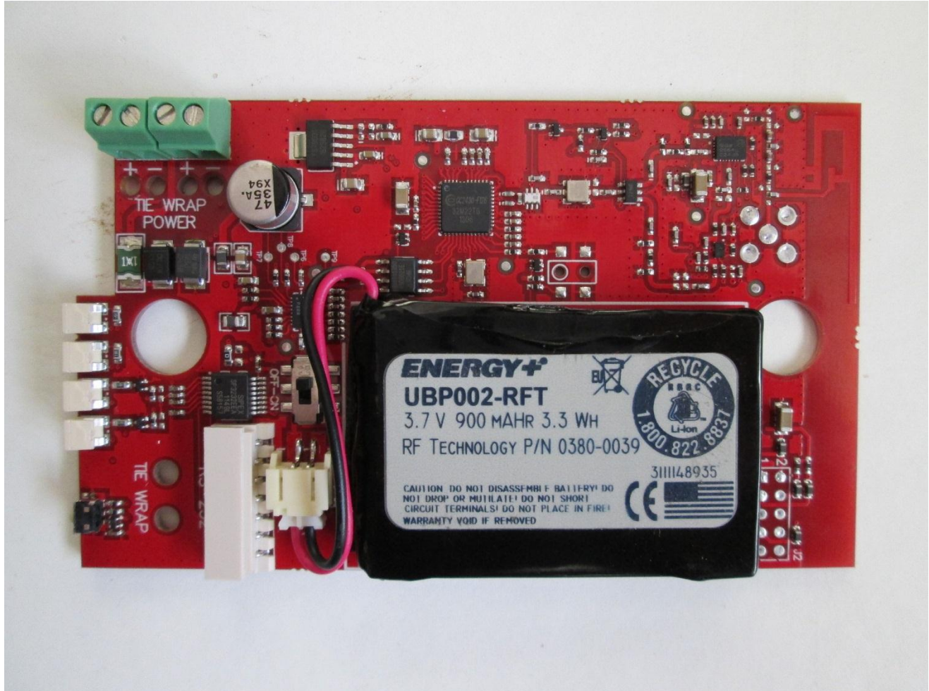
Front Circuit Board Top – with Battery
