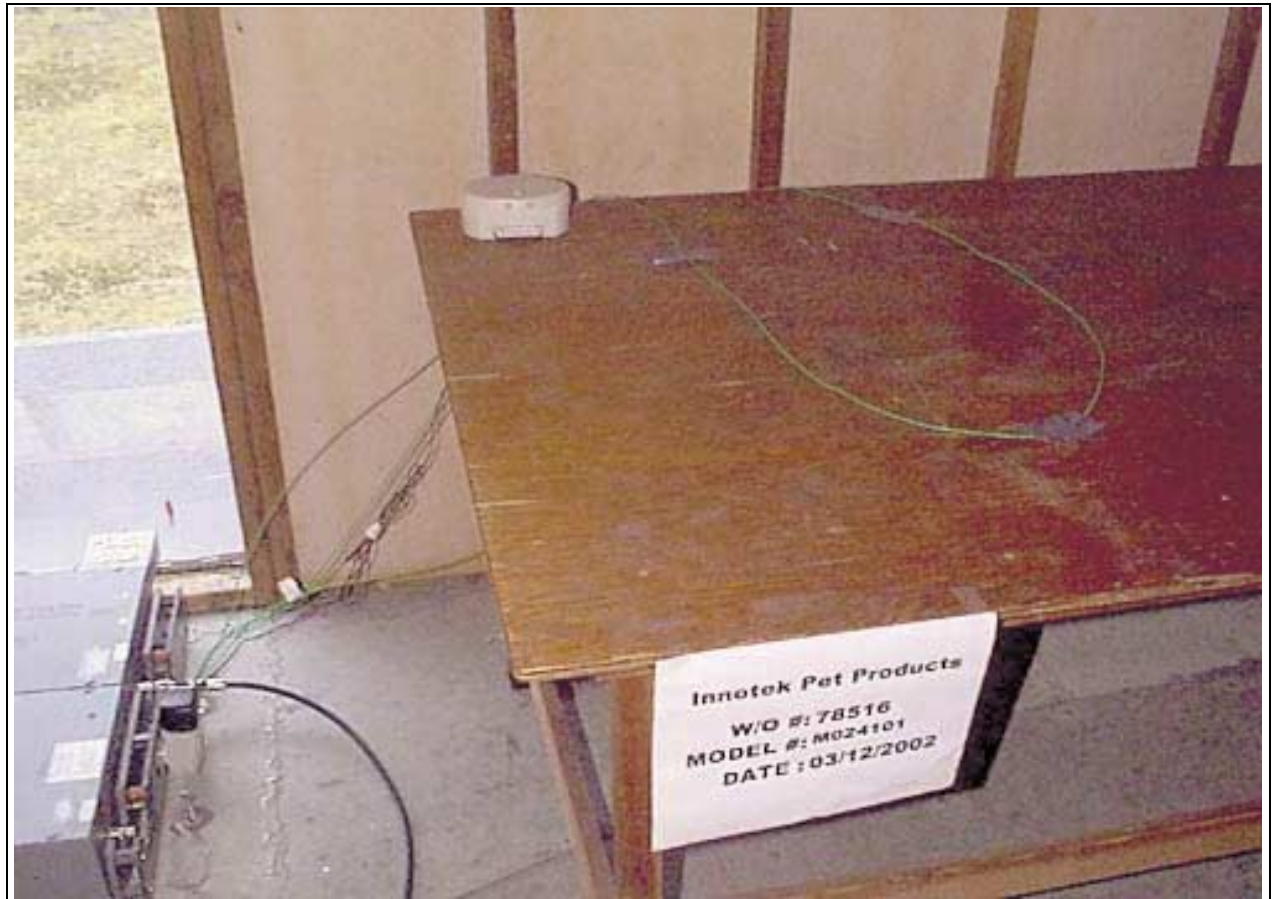
Mains Conducted Emissions - Front View
