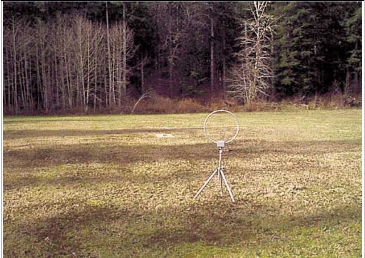
Radiated Emissions - Antenna Below 30 MHz
