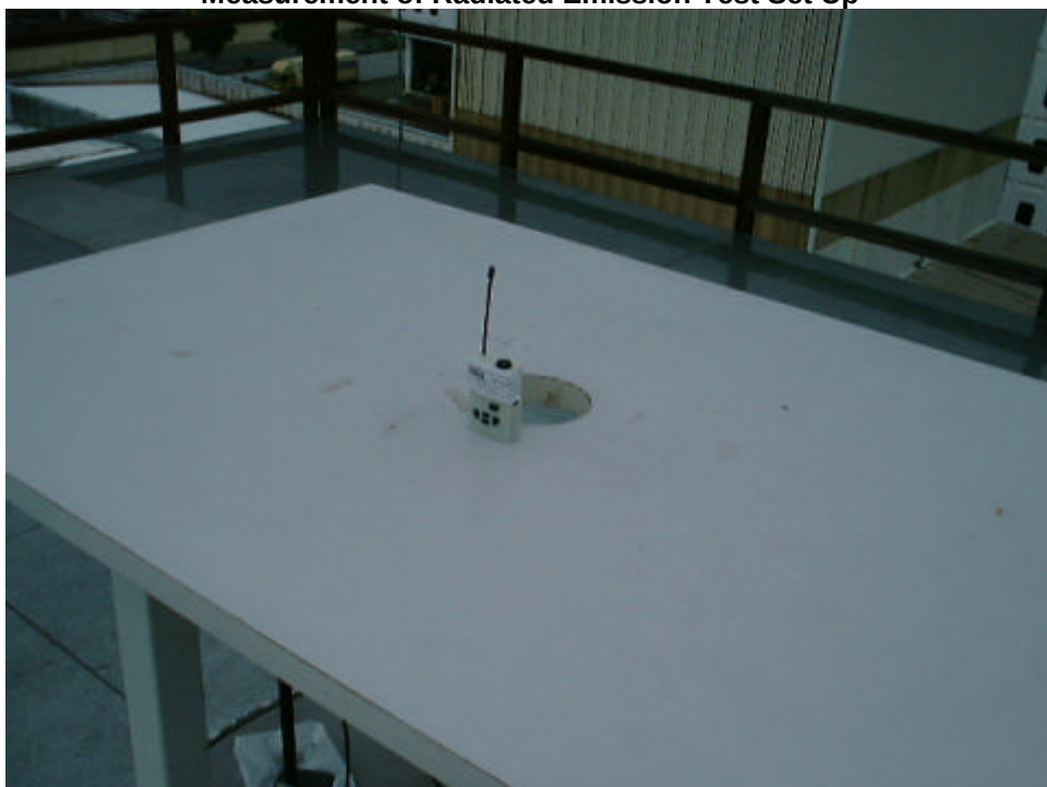
Measurement of Radiated Emission Test Set Up
