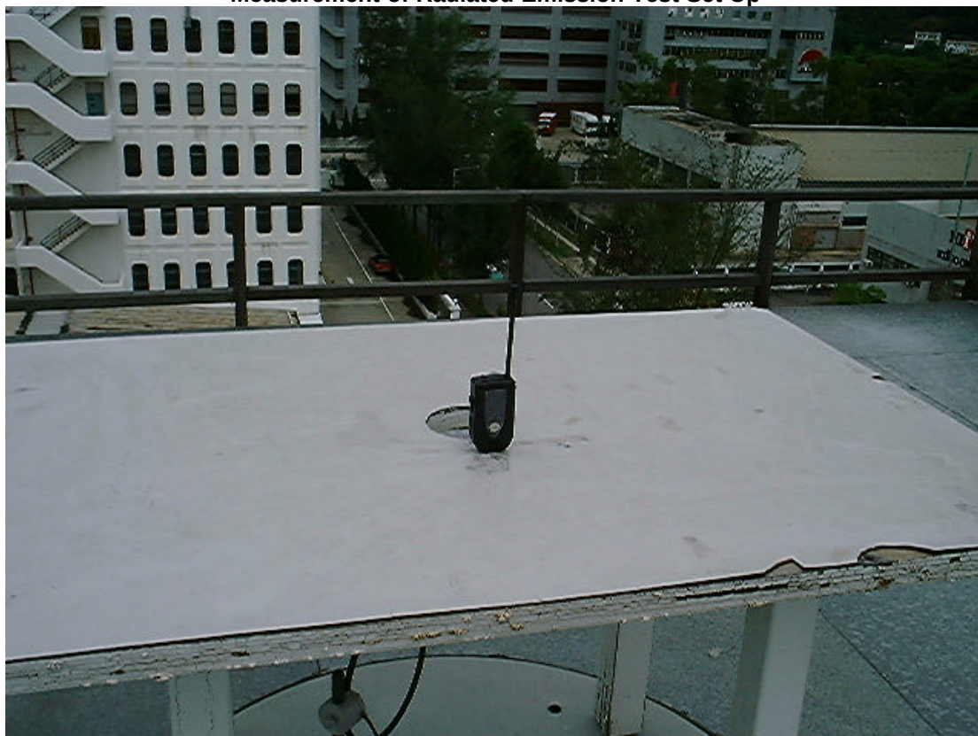
Measurement of Radiated Emission Test Set Up
