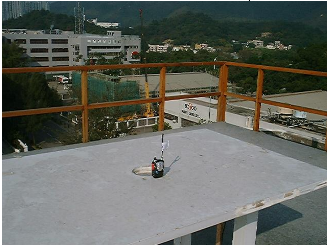
Measurement of Radiated Emission Test Set Up
