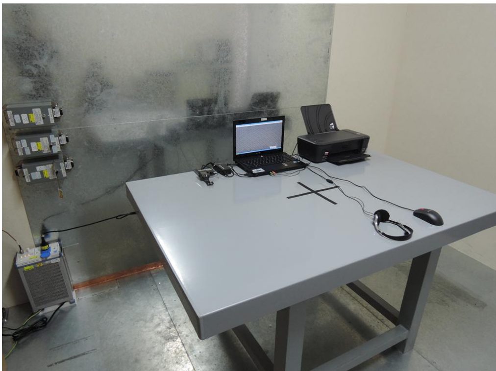
Photograph 6: Set-up for for Mains Conducted testing Front
